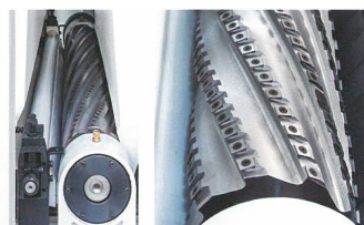
Planer carbide knives spiral along the planer head
